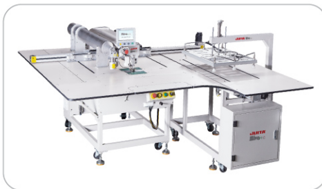
JMK8F-9AJWM Right single feeding with laser function intelligent template sewing machine Single feeding with laser function , faster and less work (specific to the equal process of cutting with sewing and put the material)
